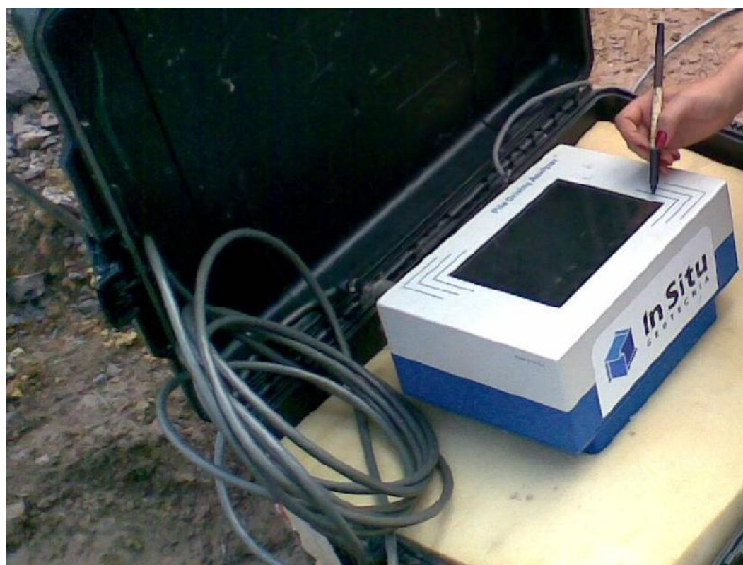
Figura 2 – Pile Driving Analyzer.
